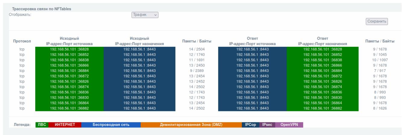
The screenshot shows a table titled 'Трассировка связи по NFTables' (Tracing connection via NFTables). The table has columns for Protocol, Source IP:Port, Destination IP:Port, Packets/Bits, and Response. It lists 14 rows of connection details, such as TCP connections between 192.168.56.101 and 192.168.56.1 on various ports. A legend at the bottom identifies network zones: LAN (green), INTERNET (red), Беспроводная сеть (orange), DMZ (yellow), IPCop (blue), IPsec (purple), and OpenVPN (dark blue).
